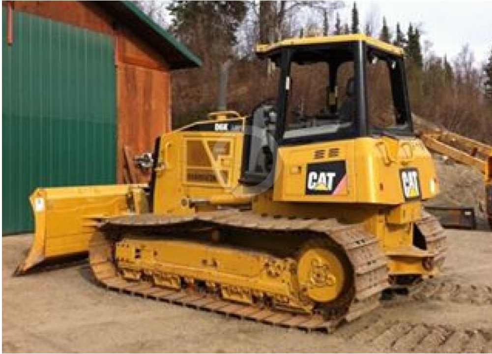
Figure 13. The D6K LGP is used mostly for reclamation and miscellaneous dirt jobs.
