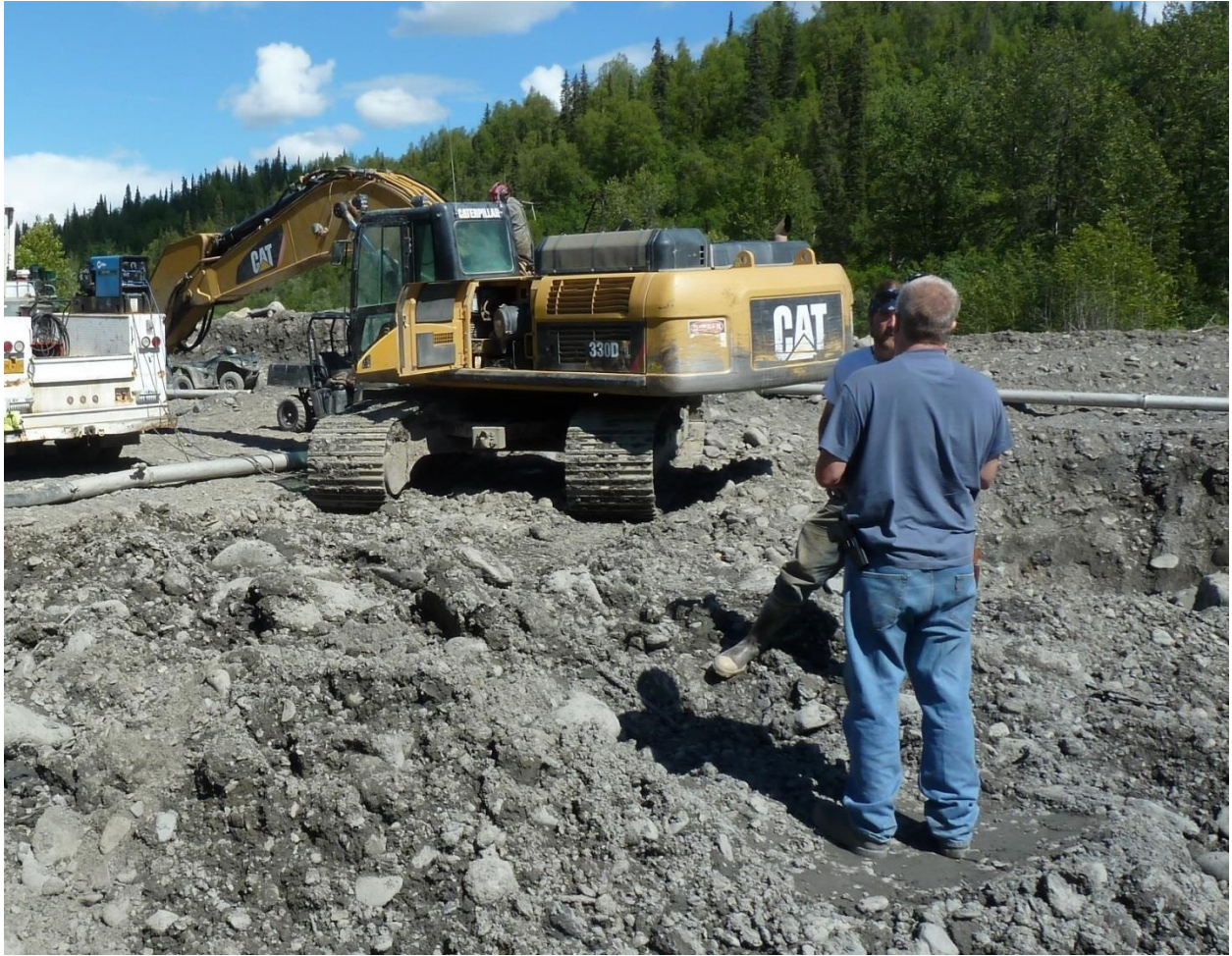
Figure 11. Caterpillar 330DL excavator which feeds the spiral wash plant.
