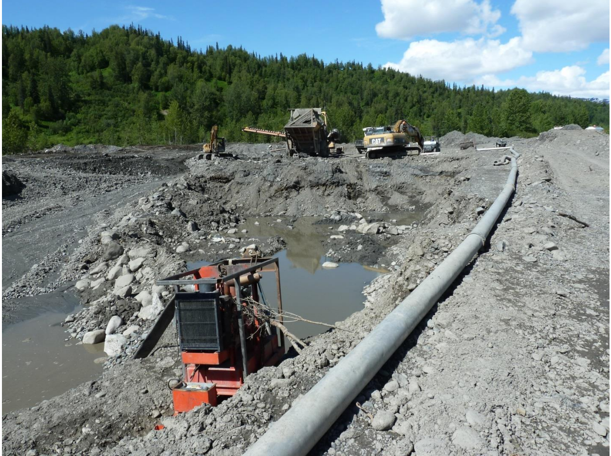
Figure 9. This shows the required equipment from left to right: the Cat 315C, orange pump, mobile spiral wash plant, Cat 330D and water supply pipe. All the heavy equipment shown in these pictures is for sale, except for the old bucketline dredge.
