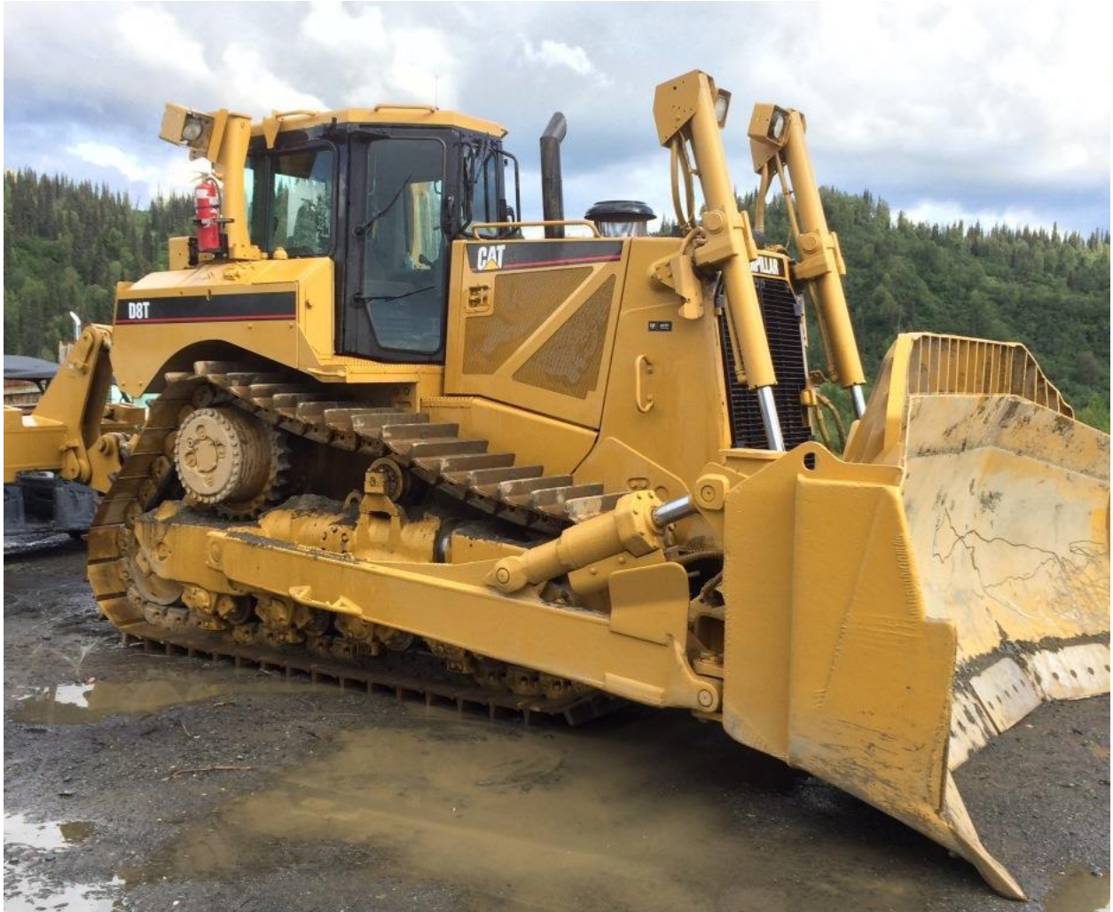
Figure 10 shows the newly overhauled and re-painted D8T that is used for stripping overburden. The undercarriage has been completely rebuilt and the dozer repainted in 2014.
