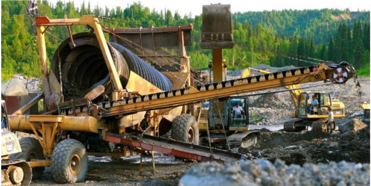
Figure 7b. Depicts the basic operation from a different angle so the stacker is more obvious. All the heavy equipment shown in these pictures is for sale, except for the old bucketline dredge.
