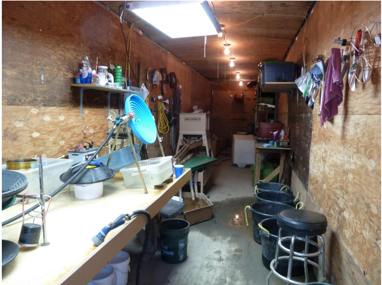
Figure 17. The clean-up trailer with Goldtron table, gold wheels, gold pans, etc. The trailer is well lite by the camp generator.
