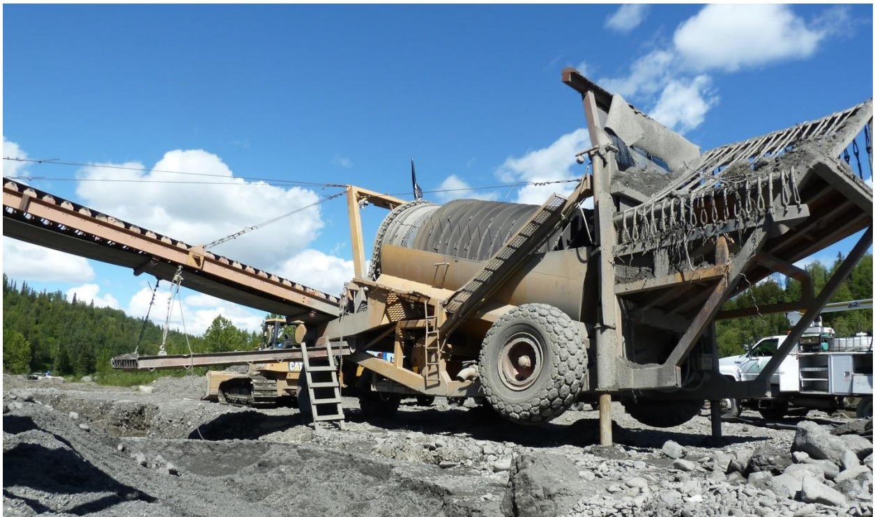
Figure 8 shows the leveled spiral trommel wash plant and stacker. Note the steel cable grizzly. All the heavy equipment shown in these pictures is for sale, except for the old bucketline dredge.
