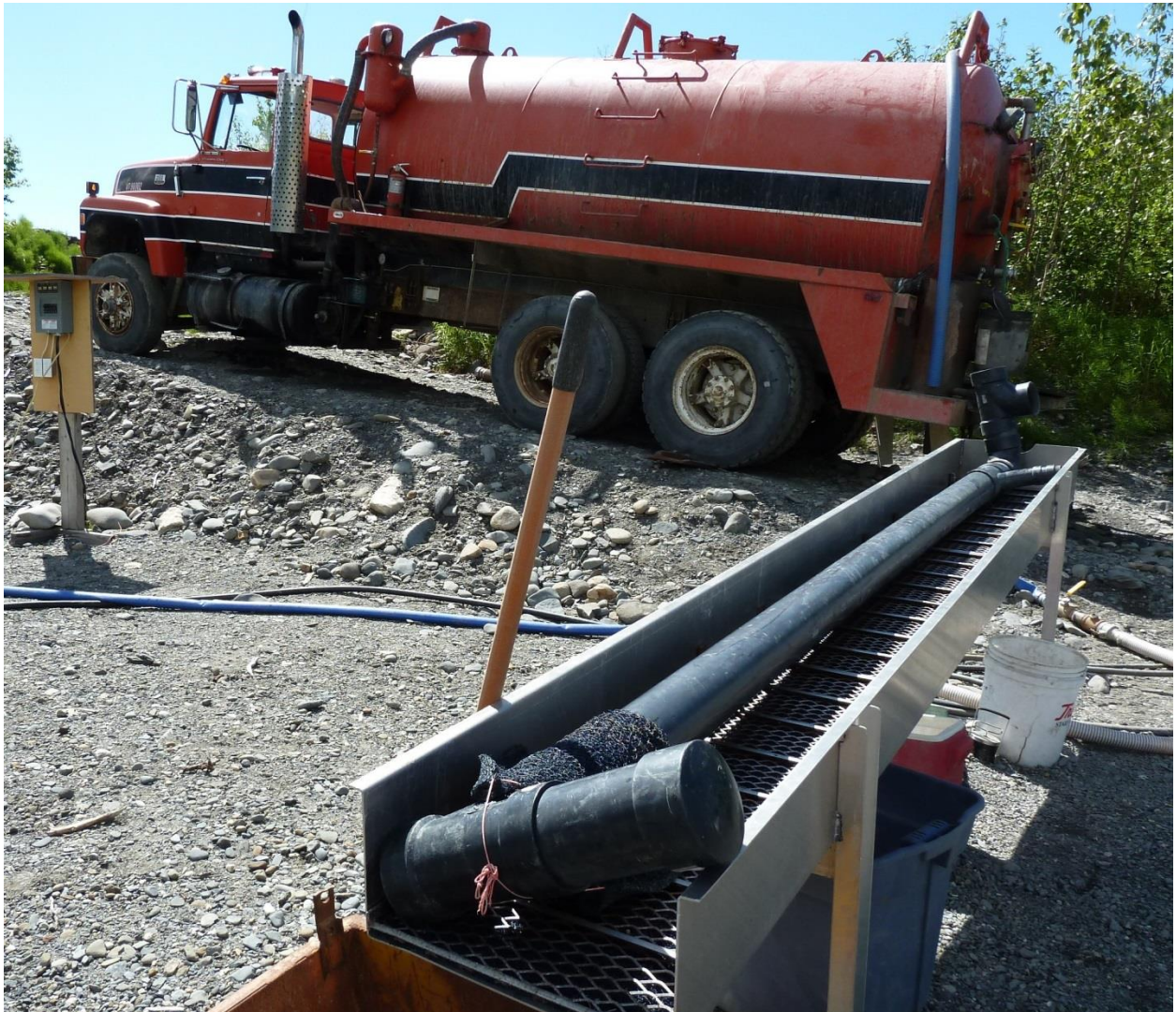
Photo 15. The clean-up (vacuum) truck and sluice box. The truck's suction pulls the concentrates out of the wash plant, then feeds it into this sluice for further concentration before going to the clean-up trailer. This method of removing the gold from the wash plant and trucking it to the cleanup facility is cutting edge.
